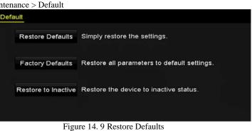
2. Select the restoring type from the following three options. **Bestore Defaults:** Bestore all parameters, except the network (including II
