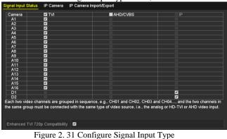
**3.** Check the checkbox of **Enhanced TVI 720p Compatibility** to enable the compatibility of TVI 720p signal input. The hint box pops up if you check the checkbox.
