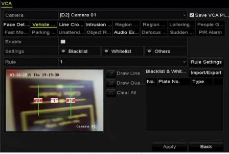
Figure 9. 3 Set Vehicle Detection
