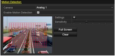
Figure 5. 13 Motion Detection- Mask
